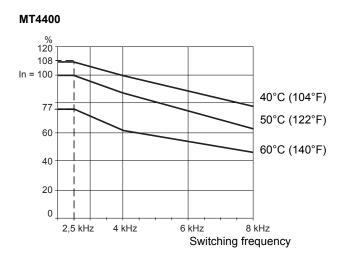
For intermediate temperatures (e.g. 55°C (131°F)), interpolate between 2 curves.
