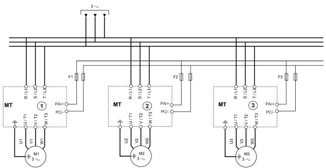
Drives (1), (2) and (3) must not be more than one size apart when they are connected in this way.
