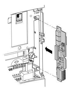
• First remove the empty option card support if it is still in place, as shown on the previous page, so that you can access the slot for the encoder feedback card.
