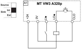
• Switch in "Source" position and use of an external +24 VDC source
