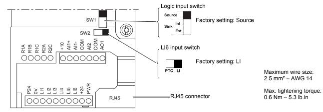
Note: The MT is supplied with a link between the PWR and +24 terminals.
