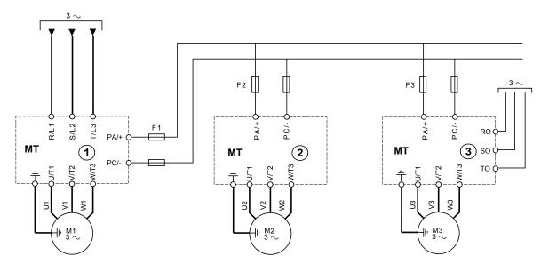
Drives (2) and (3) powered by their DC buses only do not need to have a DC choke (catalog number MT).
