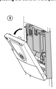
(3) Replace the control front panel over the option card (same procedure as for installing the option card, see (1) and (2))
