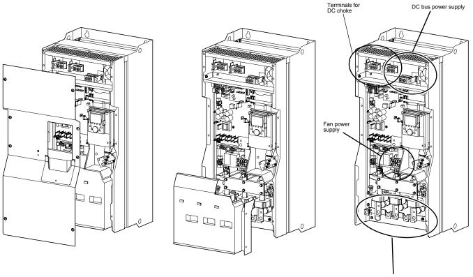
Power section AC supply Output to the motor Connections to ground Output to braking resistor (up to MT4250 rating only)
